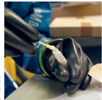
Dräger Bio-Agent Test Adding the sample to the buffer solution
