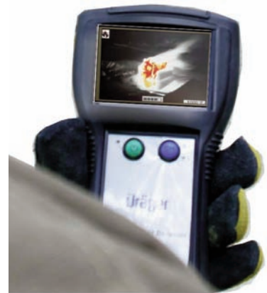
Dräger UCF1600/3200 Handheld Receiver For remote viewing of Dräger thermal imaging camera operations
